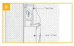
Cut Top Cap to size. Place the back lip of the Top Cap into the groove on the top of the SlatWall panel then snap the bottom lip onto the panel. Both vertical J Trims should overlap the Top Cap at both ends.
