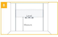
Measure from the floor. Mark the desired height of the bottom of the SlatWall area, extending a line the entire installation width using a level.
