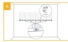
Using tin snips, cut the 1/2" J Trim to the horizontal length. Align trim bottom with the horizontal height mark and fasten at each stud except for the studs at either end.
