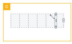
For drywall surfaces, use a stud finder and a level to locate and mark the entire length of each stud in the installation area from the top to bottom.
