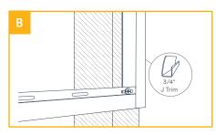
Cut two pieces of 3/4" J Trim to vertical length. Place the vertical J Trim over the horizontal J Trim where they meet, and screw into the stud where both flanges overlap.
