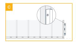
Ensure vertical J Trim is straight using a level and temporarily fasten the very top to hold it in place. Repeat for the other vertical J Trim.
