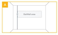
Each panel must start/finish on a stud. If the installation surface is drywall, locate and mark the first and last studs using a stud finder.
