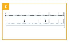
Insert the next panel into the J Trim channels on both ends and slide it down to the previous panel.
