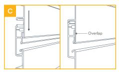
Securely interconnect the two panels by applying gentle pressure until a "snap" is felt and heard. Proper interlocking of panels is shown above.
