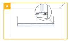
Insert the first panel between vertical J Trims and slide it down until seated in the bottom J Trim. Screw through the flange into each stud, leaving 1/16" min. gap under screw heads. At both ends, screw through the overlapped flanges.
