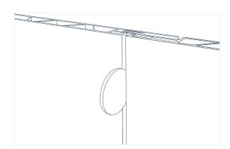
At Panel Ends – Increase the spacing allowed at the end of panels from the typical ¼" to 3/8". If you are joining panels at the ends, the H Channel Snap-In trim kits have a wide face trim and are perfect for covering the extra gap required.
